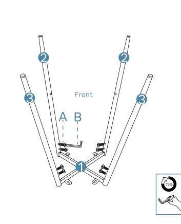
Attach 2 x legs (3) and 2 x legs (2) to frame (1) as shown and secure with 8 x bolts (A). Tighten with an Allen Key (B).
